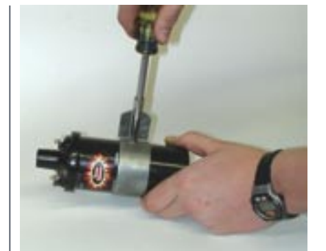
10. The beauty of the high-output Flame-Thrower coil is that it exactly resembles a stock OE coil and fits directly in the original bracket. For a stealth look, just remove the Pertronix decal.
