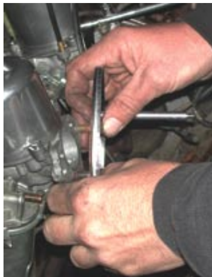
1. We installed the individual chrome air-filter assemblies next by attaching the base and new gasket.
