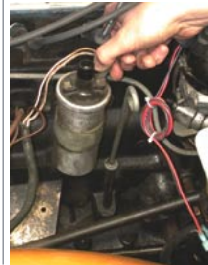
8,9. At this time we deviated from the Ignitor installation instructions to install the Flame-Thrower coil. Craig unbolted the stock coil after removing the wire harness from the positive side of the coil.
