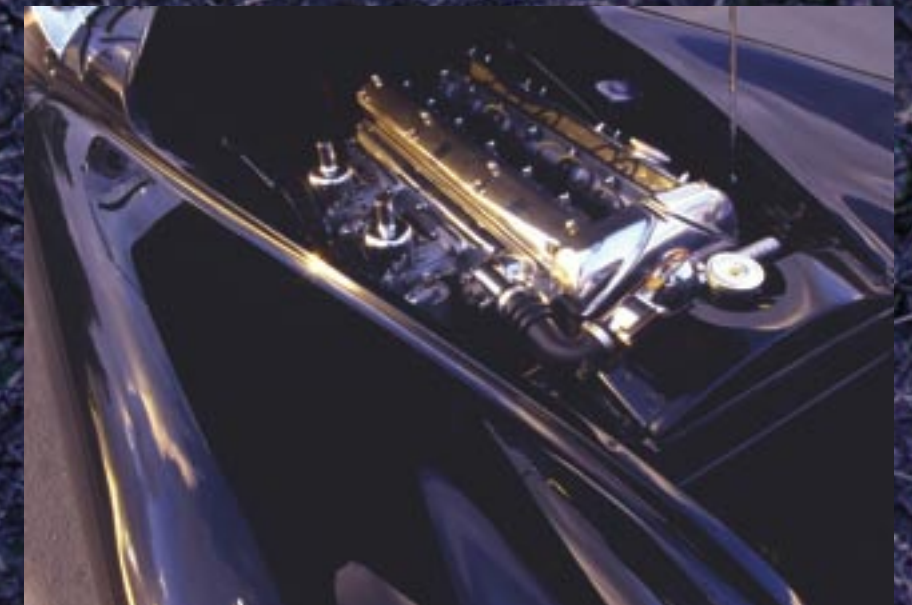
Originally intended as simply auto-show window-dressing for a new engine, the XK120 rocked the automotive world at its 1948 introduction. Its 3.4L I-6 powerplant was the first mass-produced DOHC/hemispherical-head design, and its 160 hp propelled the roadster to a 120-plus-mph top speed.
