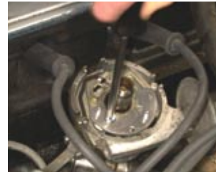
4. We wiped the distributor plate with a rag, then fastened the Ignitor adapter plate with the single countersunk flathead screw.
