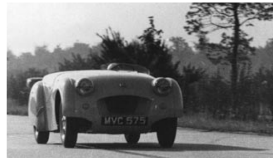
Ken Richardson established a world speed record for two-liter production sports cars of 124.095 mph. To reduce drag, the seat was removed and Ken hunched down on a cushion.
