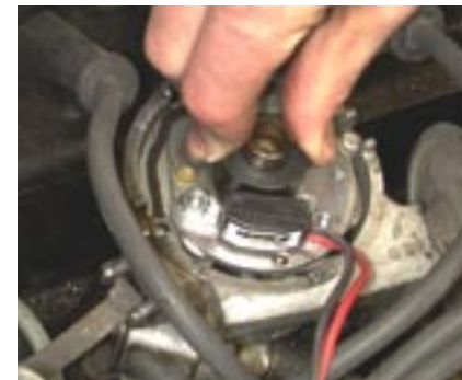
6. Craig then slid the magnetic sleeve over the distributor shaft and points cam. Rotate it back and forth until you feel it line up, then push it all the way down.
