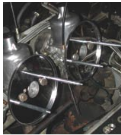
2. Here are the two bases bolted to the carbs and awaiting the filters and tops. The bases use studs so that chrome acorn nuts can be used to hold the lid on. This makes for a clean look when complete.
