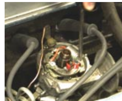
3. Next, remove the points, condenser and grommet that fits in the housing of the distributor. The points and condenser simply unscrew from the plate.
