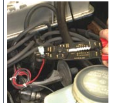
11. With the coil bolted back in place, we found that the Ignitor wire leads needed larger connectors for the spade-type connections on the coil. We snipped off the old ones and crimped the appropriate connectors onto the Ignitor wires. At this time, you could also trim them to the proper length.
