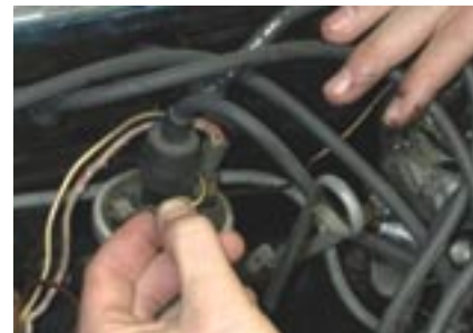
2. Disconnect the points wire from the negative side (-) of the coil.
