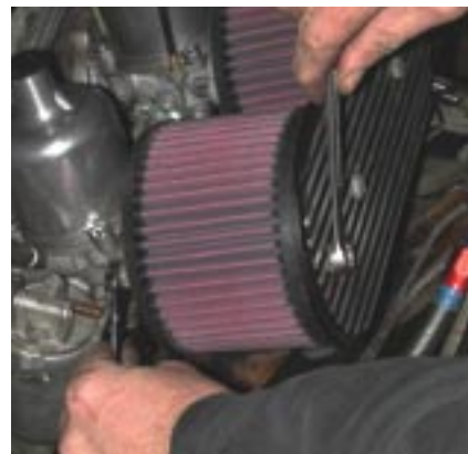
3. You'll need two wrenches to get on the bolt and the nut. Again, do not overtighten as this can damage the filter, the top, or the base.
