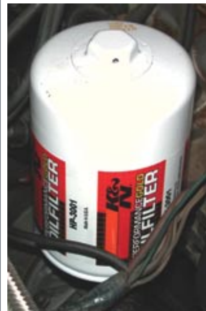
While we were at it, we installed a new K&N Performance Gold oil filter in place of the stocker. The Performance Gold features a unique design that outperforms OE-style paper oil filters for added protection.
