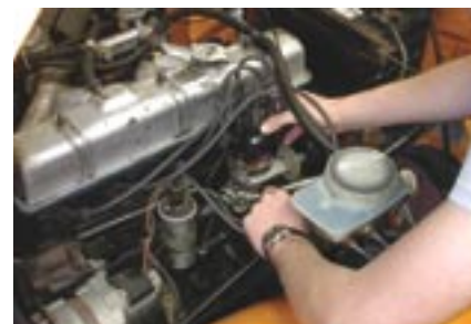
1. The first step is to remove the distributor cap and push it out of the way. Do not remove the spark plug wires.
