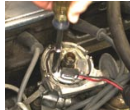
5. The Ignitor ignition module slides down over the two studs on the adapter plate and is tightened in place by nuts with integral star washers.
