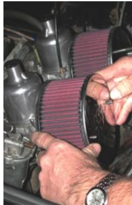
3. The filter and lid fit on the base as shown. Be sure that the filter fits flush into the base to ensure a good seal.
